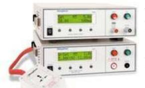
All models in the 2900 series can be interconnected to the 2630 to form a complete entry level system, which will perform the most commonly specified electrical safety tests including AC and DC Dielectric Withstand, Insulation Resistance and Ground Bond in a single Device Under Test (DUT) connection. The system is a cost-effective way to test to safety agency standards that require high voltage test of insulation and high current tests of the protective ground circuit.
